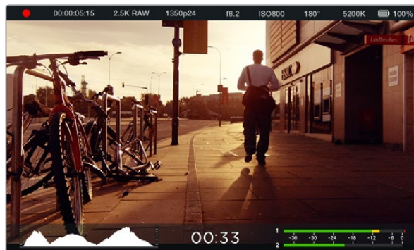
On screen meters and status strip on the Blackmagic Cinema Camera. Swipe up from the bottom of the screen to reveal the meters.
