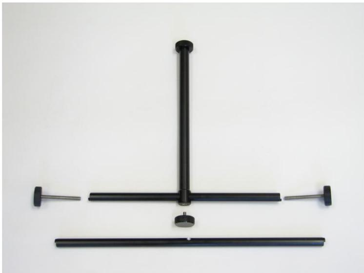
Remove the counterweight screws that are on the present bar you are using and set them aside. Remove the horizontal bar screw and set it aside. Slide out the horizontal bar. Insert the new bar and line up the tapped hole through the bottom of the T-joint. Screw the horizontal bar screw back in to secure the bar. Re-insert the counterweight screws on the new bar.
