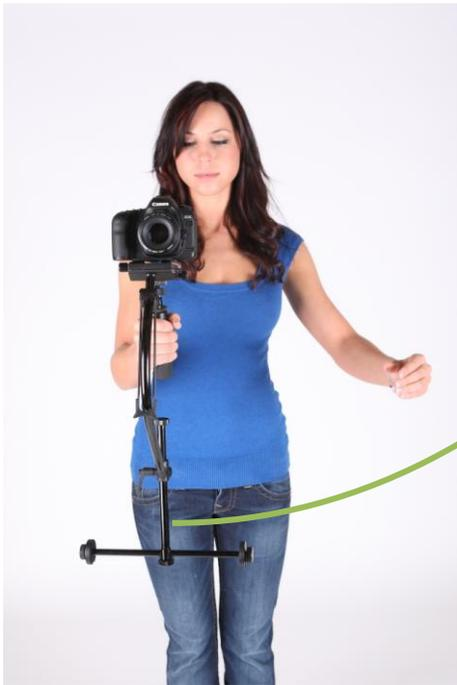
Note that to get a good drop test the stabilizer should be at least roughly in balance horizontally. If the Blackbird wants to rotate on its pan axis when you release it, or if it leans to one side instead of dropping all the way down this is a sign of horizontal balance being off. So with the rig in any bottom heavy condition first do a horizontal balance (see horizontal balance below) before checking drop time.
