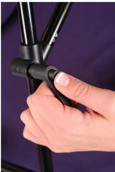
Tighten the T-bar clamp by turning it clockwise to secure the T-bar. You can change the end position of the T-bar clamp (without loosening it) at any time by pressing on the button and pulling it out and then rotating it to the desired position.
