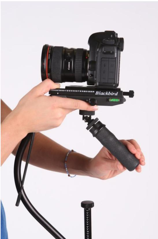
Observe the freely swinging handle to see the amount of friction being added. To do this support the Blackbird with one hand under the camera stage and lift the gimbal to about a 45 degree angle and release it. With no friction it should pendulum about 4 to 6 times before coming to rest. As you adjust more friction and drop the handle you will see it come to rest after fewer and fewer pendulum swings. With a very high friction adjustment the handle will just overshoot vertical and stop.
