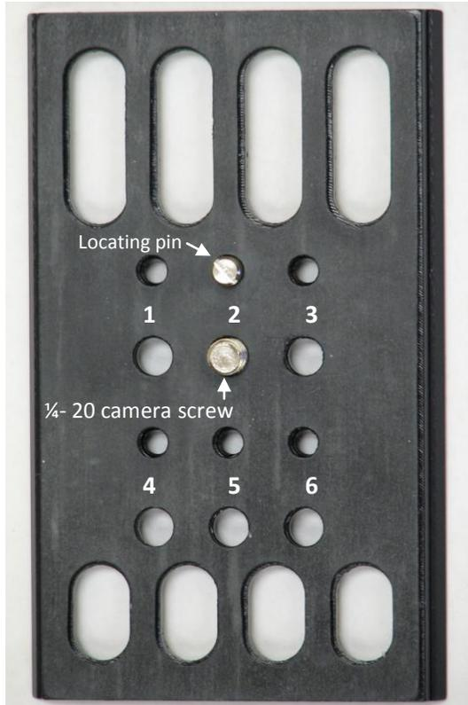
Place the 1/4-20 camera screw in the hole that you think will locate the center of gravity of the camera directly over the gimbal. Or just start with the #2 hole in the middle of the camera mounting plate and check balance. The locating pin screws into the appropriate hole.
