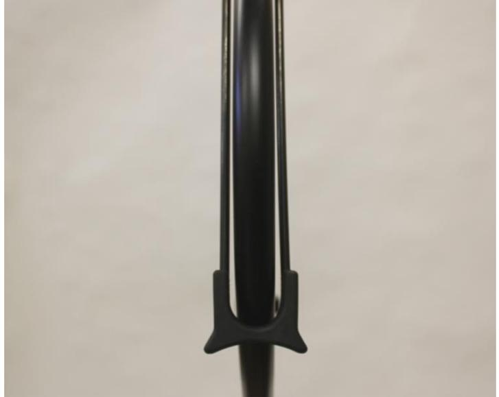
The resting stand should be folded down for normal flying and flipped up to set down the Blackbird.
